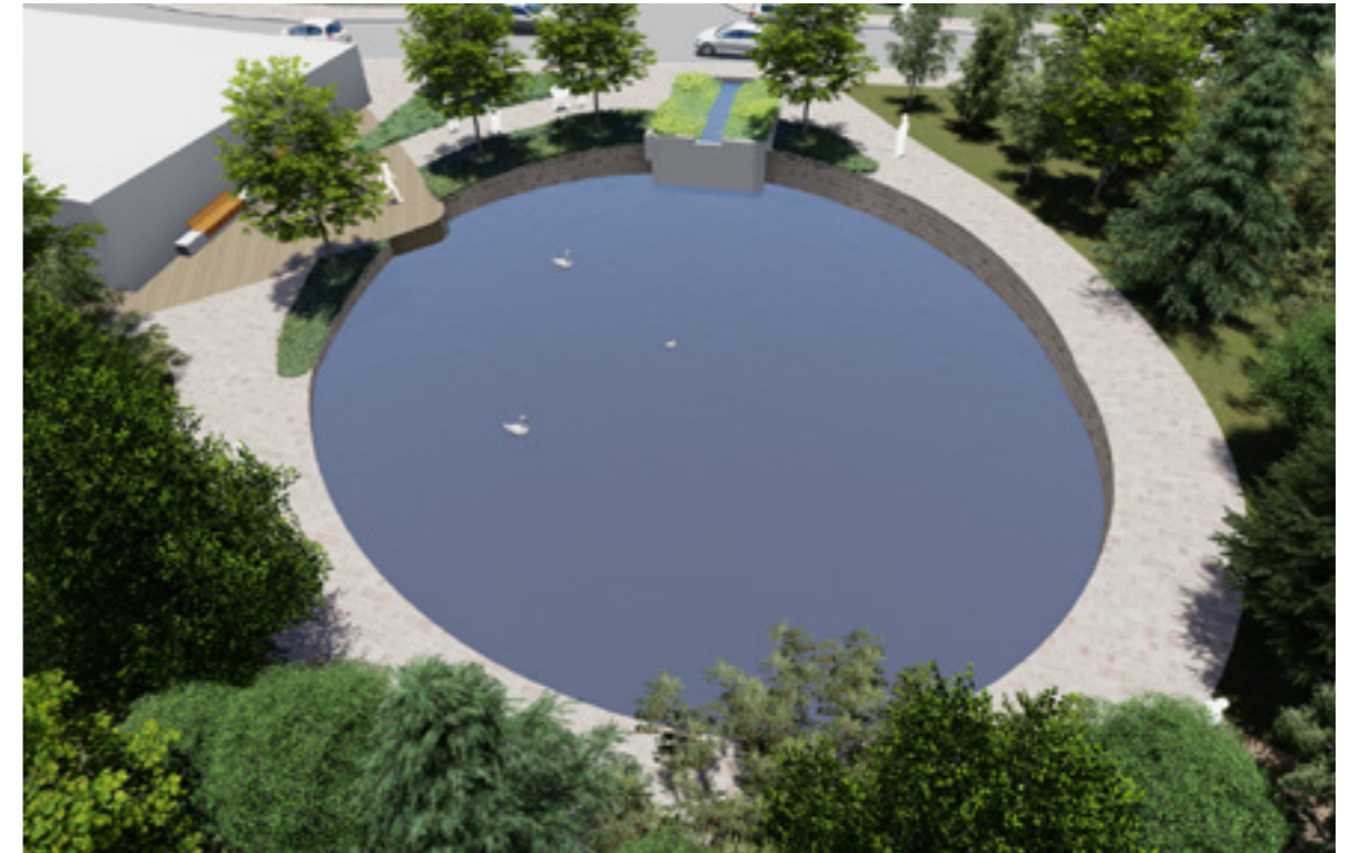
Illustrative view of balancing pond for attenuation
